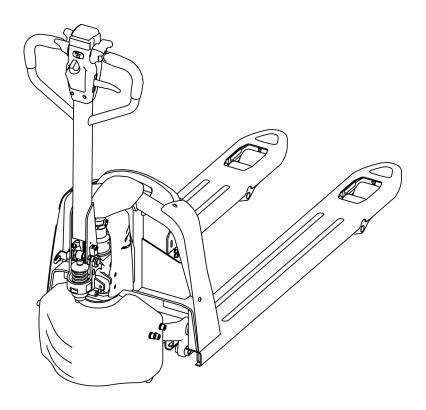
CBD15/20 Type is a Electric pallet truck. It adopts the advanced structure such as ring rod lifting system and DC controller, at same time it is equipped with high quality motor, traction battery and pump station motor. It has the characteristics of superior performance, convenient operation, flexible steering, reliable braking, good dynamic performance, less noise, less pollution and beautiful appearance.
