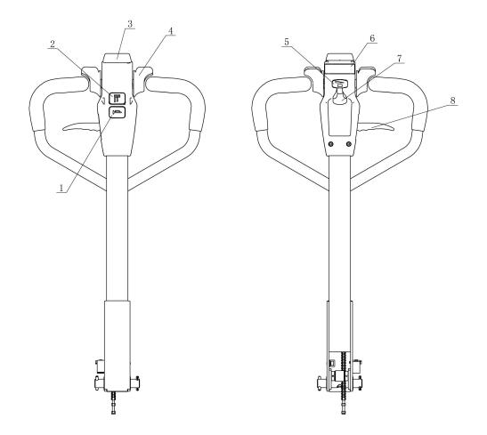
1. Horn2..Switch for lifting3Belly switch4.Switch for driving5.Electricity meter6.Tortoise Speed switch7.Key switch8.Switch for lowering
