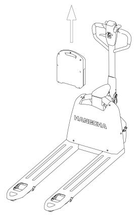
D: Insert the new battery into the battery mounting solt.
