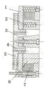
Braking principle diagram
