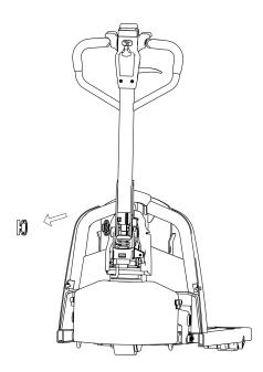
C: Pull up the battery and pull the battery out of the car.
