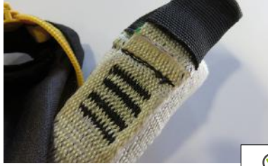
• Absorber has sustained an impact load; absorber has started to tear
