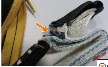
• Absorber has sustained an impact load; absorber has started to tear
